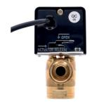
Power supply/ Frequency: 230 V AC/ 50 - 60 Hz Power consumption: 7 VA Kvs coefficient: 6.5 m³/h Operating condition of actuator: 0 - 60°C Running time (motor): 18 s Running time (return spring): 5 s Degree of protection: IP 20
